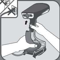
**EN** Unlock and remove the water tank.
