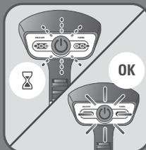
**EN** Wait until the light stops flashing. When the light is steady the appliance is ready to use.
