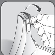
**EN** Remove the water inlet stopper.
