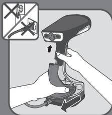
EN Unlock and remove the water tank.
