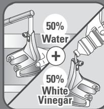
EN Fill the water tank with 50% water and 50% white vinegar.
