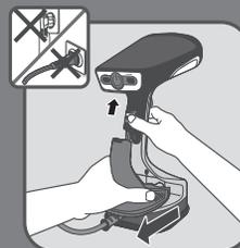
EN Unlock and remove the water tank.
