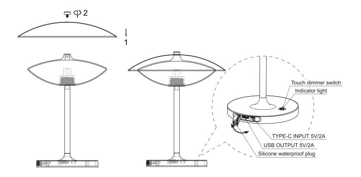
When pressing the on/off indicator, the light will dim up/ down. During charging, there will be a green indicator flash. After fully charged the green indicator will keep lighting on. Blue indicator light means that the lamp is charging other devices. Blue light flashes means the lamp needs to be charged.
