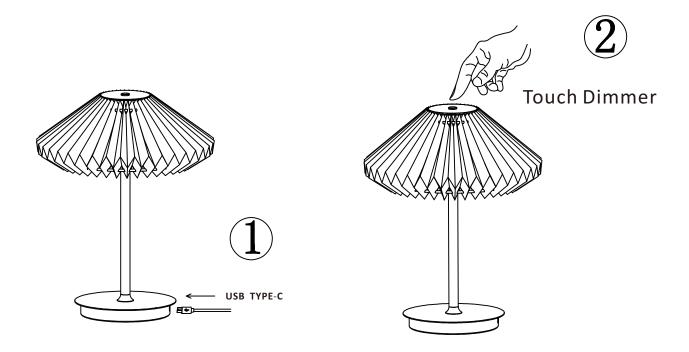
When pressing the on/off indicator, the light will dim up/ down. During charging, there will be a red indicator lighting. After fully charged it will light green.
