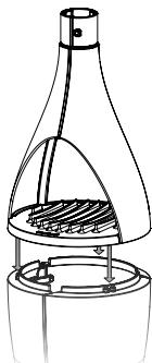
3. Place the firebox on the plinth such that the shadow edges on the plinth and firebox are flush.
